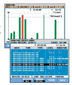
The System-Monitor overview screen gives instant insight into whether the voltage, harmonics, flicker, frequency and the number of dips and swells fall outside the set limits. A detailed list is given of all events falling outside the set limits.
