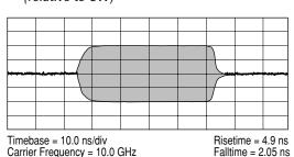
Typical pulse modulation envelope illustrates the fast rise and fall times, excellent flatness, and pulse fidelity of the 83731B/83732B.
