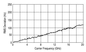
Typical residual FM measured in 50 Hz to 15 kHz bandwidth, CW mode, with high-stability timebase, Option 1E5
