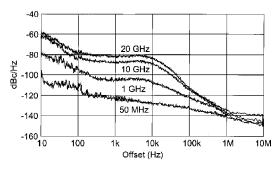
Typical single-sideband phase noise at 50 MHz, 1 GHz, 10 GHz, and 20 GHz, 25°C, CW mode. Offsets less than 100 Hz require the high-stability timebase, Option 1E5.
