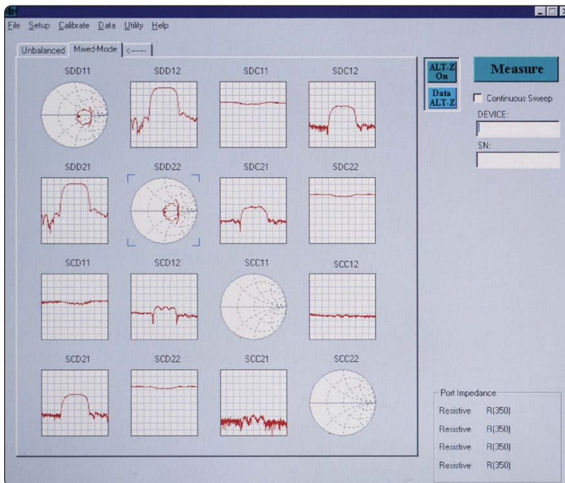
Example showing mixed-mode S-parameters of a SAW filter.
